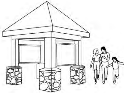
Figure 7 – Preliminary kiosk design with Shade structure on piers and sign panels on three sides. Each panel with information on each side
